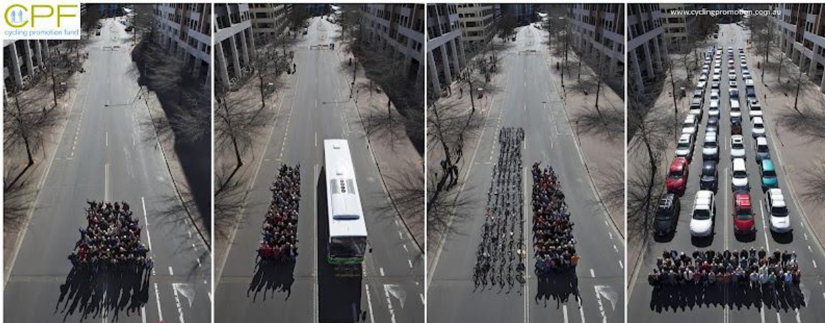
Figure 1: Road space required to move 69 people by walking, bus, bicycle and car, Canberra, September 2012
